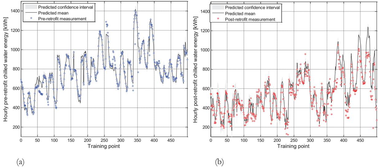
**Figure 1** (a) Hourly pre-retrofit chilled-water energy use predictions (black line) compared with pre-retrofit measured energy use (blue dots) and (b) hourly post-retrofit chilled-water energy use predictions (black line) compared with post-retrofit measured energy use (red dots)
