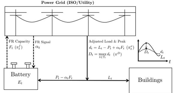
Fig. 2: Interactions battery, buildings, ISO, and utility.
