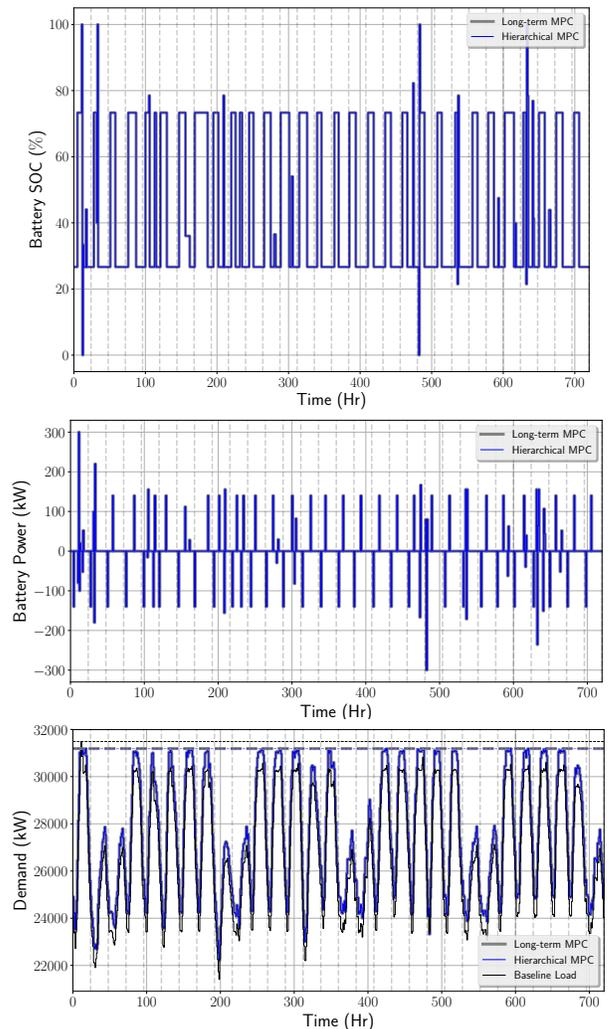
Fig. 4: Comparison of battery SOC (top), battery power (middle) and demand (bottom) policies.
