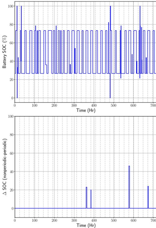
Fig. 5: SOC policy without periodicity (top). Difference of SOC policies with and without periodicity constraints (right).
