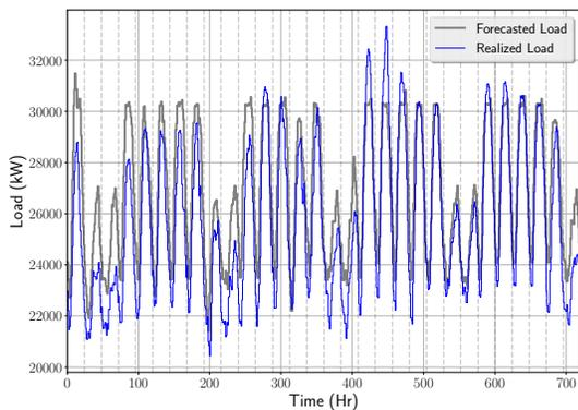
Fig. 6: Forecasted and realized load profiles.
