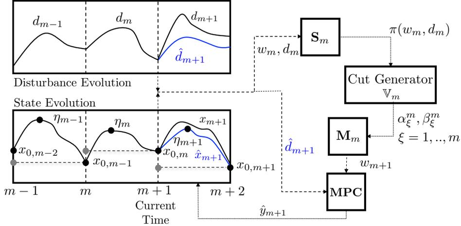
Fig. 1. Sketch of hierarchical scheme using cutting planes.
