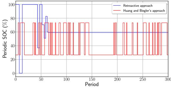
Fig. 7. Comparison of evolution of periodic SOC resulting from the retroactive approach and Huang and Biegler's proactive MPC approach [13].
