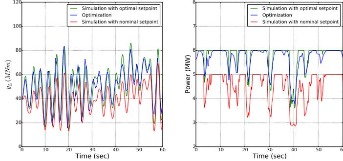
Fig. 4: Power and load profile instances at 15 m/sec.
