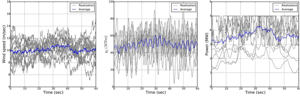
Fig. 3: Wind, load, and power profiles for mean wind speed of 10 m/s.
