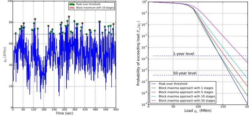
Fig. 2: Extreme loads (top) and extreme value distributions (bottom) for peak over threshold and block maxima approaches.
