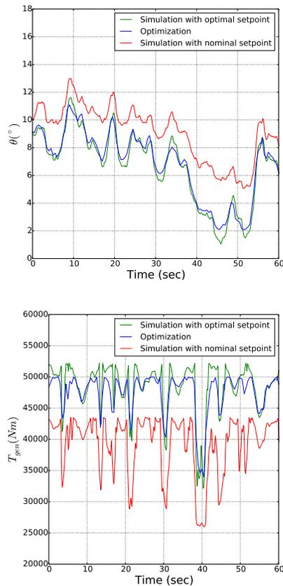
Fig. 7: Pitch angle and torque 15 m/sec.
