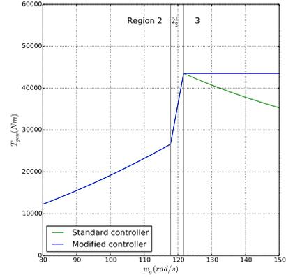
Fig. 1: Standard and modified torque control laws.
