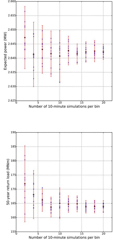
Fig. 4: Expected power confidence levels (top) and 50-year characteristic load (bottom) confidence levels.
