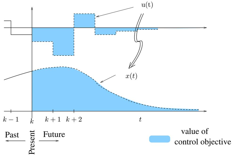
Figure 1: MPC: prediction horizon and objective function.
